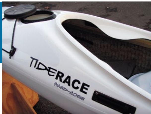
The compartment forward of the cockpit provides safekeeping and easy access for small items.
